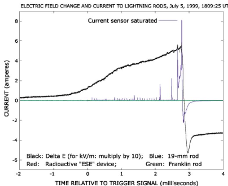
**Figure 3:** Plots of the electric field changes and of the currents that flowed from three lightning rods mounted on 6-m high masts above Kiva II on South Baldy Peak when lightning struck a 12.7-mm diameter blunt rod located 42-m
