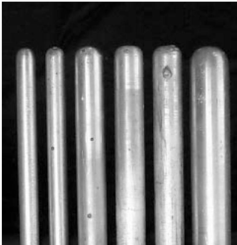
**Figure 1:** Photograph of six blunt aluminum lightning rods, each of which has been struck by lightning. The two rods on the left were 12.7-mm in diameter, the rod on the right was 25.4-mm in diameter and the diameters of the other rods were 19 mm.
