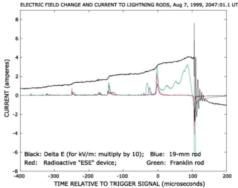
**Figure 4:** Plots of the electric field changes and of the currents that flowed from three lightning rods mounted on 6-m high masts above Kiva II on South Baldy Peak when rocket-initiated lightning struck a pine tree located 33-m NNE of Kiva II (August 7, 1999).
