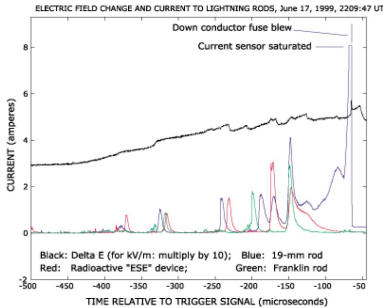
**Figure 2:** Plots of the early electric field changes and of the currents that flowed from three lightning rods mounted on 6-m high masts above Kiva II on South Baldy Peak when lightning struck the 19-mm diameter blunt rod (June 17, 1999).
