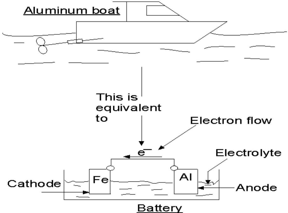
For galvanic corrosion to occur, there must be an electrical circuit. This means there must be a path for the electrons to travel between the two dissimilar metals and there must be a path through the electrolyte for the ions to travel. Additionally, the chemical reaction at the cathode usually requires the presence of oxygen in the electrolyte.
