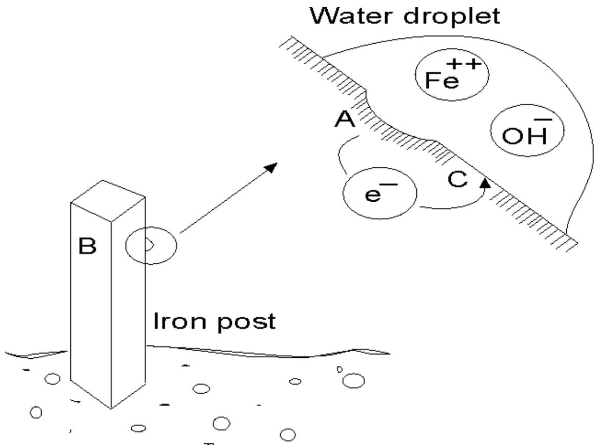
If they can travel towards one another, such as through the water (in this case termed the **electrolyte**), they will. In the case of the steel and hydroxyl ions, they combine to form rust. The "iron post in the ground" has corrosion occurring even though it is one metal.
