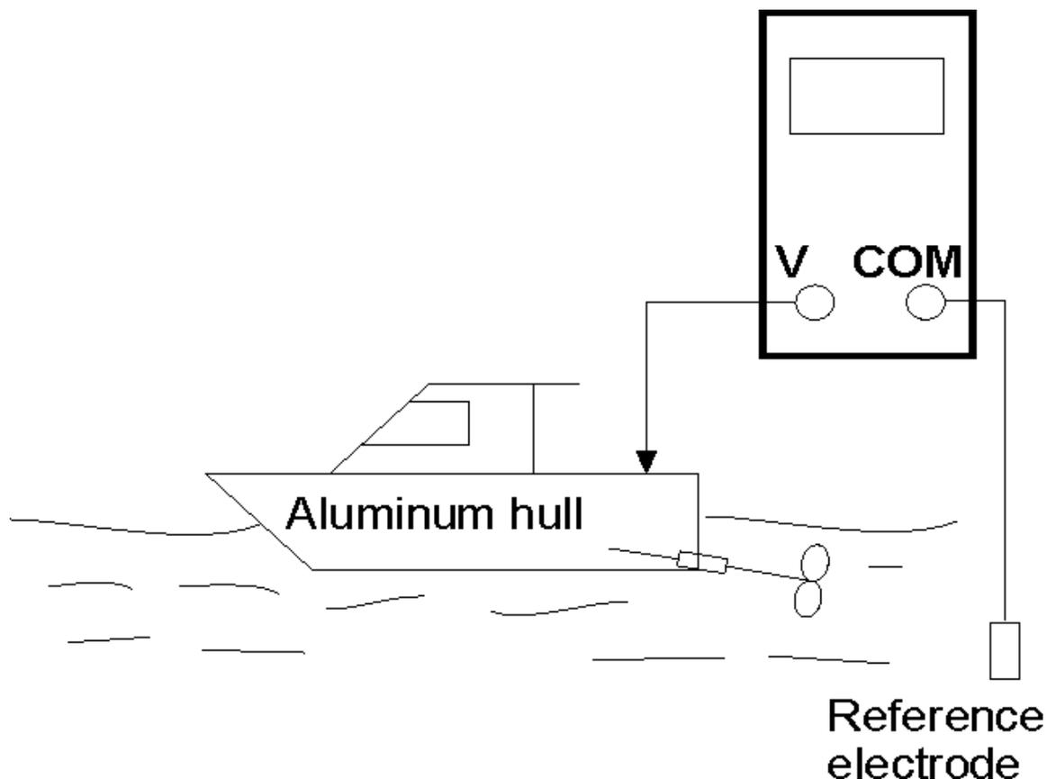
Place the reference electrode (silver silver chloride) in the sea water, and connect the multimeter red lead to the hull. If the reading on the multimeter is between -850 mV and -1100 mV, then the zincs are working and your boat hull is protected. You should then repeat the test with the out drive.
