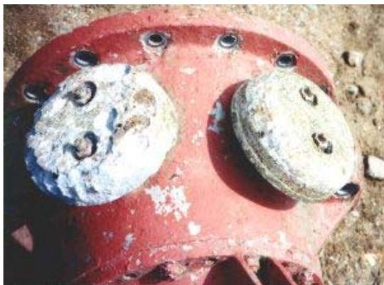
How do you check if an anode is working? If the boat is in the water, then looking to see if the anode is corroding is one way. This is not completely fool proof as the anode may still be functioning correctly but the protection level may be insufficient to prevent corrosion.
