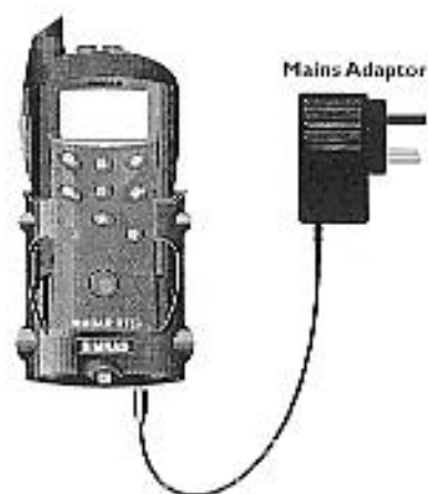
Fig 2 - Charging from AC source (110v/220v)
