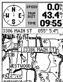
Creating a waypoint using the panning arrow.
