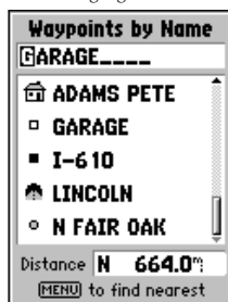
Waypoints By Name List. Use the ROCKER keypad to enter the first characters of the waypoint name or scroll through the list.
